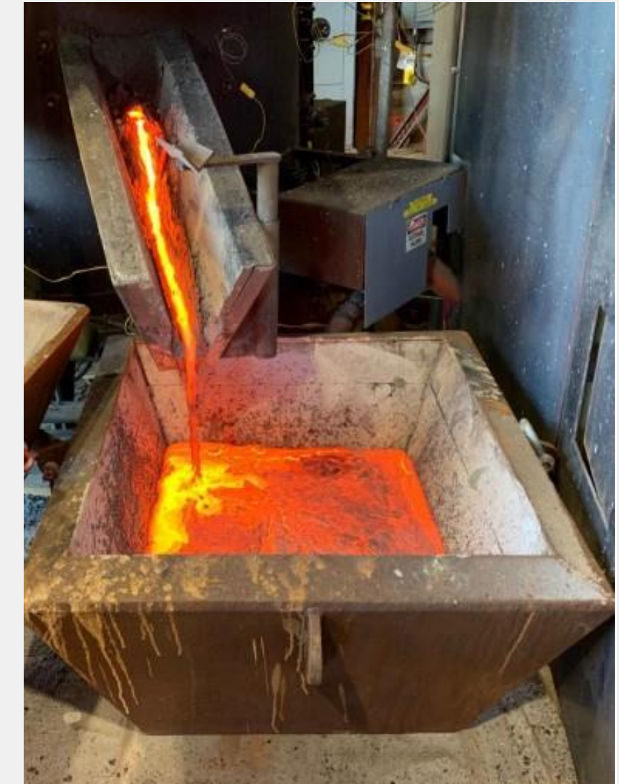
Matte pour post converting. End-product is NiCuCo matte, 80% Ni+Cu.
